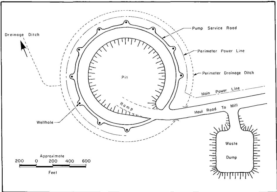
Figure No. 5 Typical Well and Ditch Arrangement
