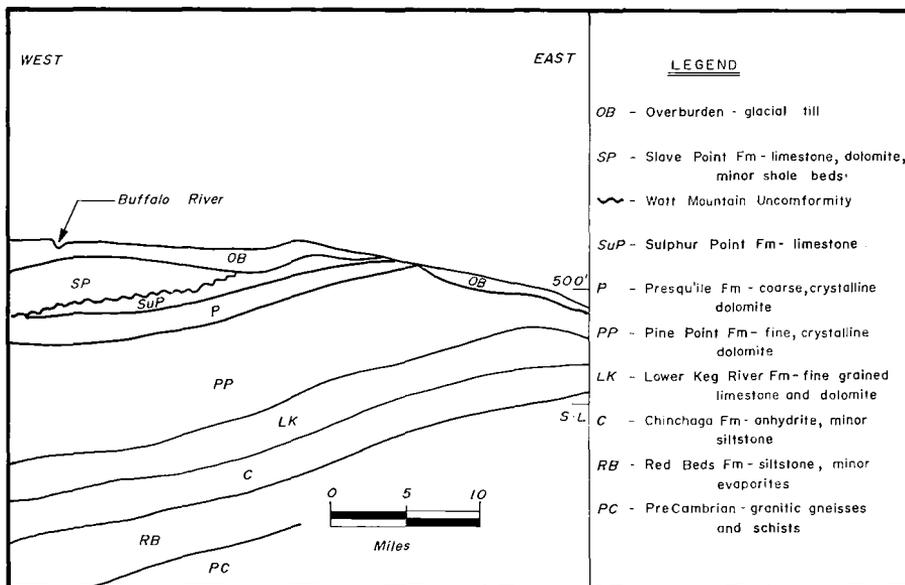
Figure No. 4 Generalized Geological Section
