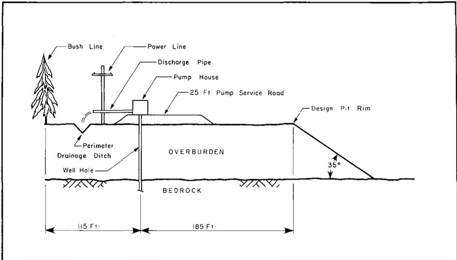
Figure No. 6 Section of Typical Pit Rim Arrangement
