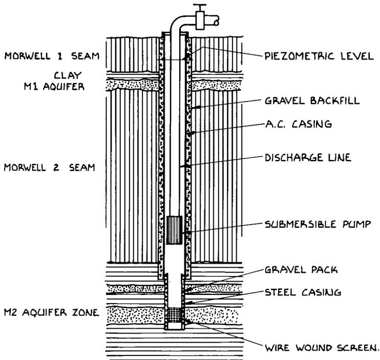
Figure 7 - M2 Aquifer Pumping Bore
