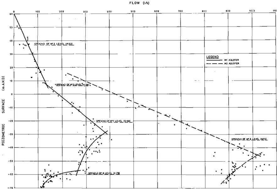
Figure 6 - Relationships Between Piezometric Level and Flow
