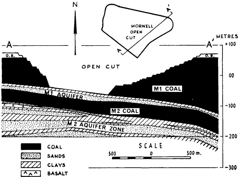
Figure 2 - Morwell Open Cut Section
