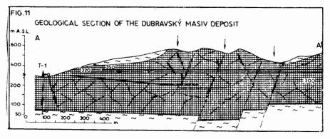
The ground water formation and accumulation is first of all related tp fissuring and karstification. Magnesites have most intensively undergone karstification and karst phenomena developed there in to a higher stage (merokarst). In rare cases, some horizontal karst phenomena (and extensive gallery and cavern system being up to 500 m long) are here present, too.
