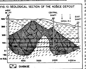
The predominant part of the deposit lies beneath the erosion base and due to the tectonic pattern, karstification and possible direct rainfall infiltration it is characterized by intricate hydrogeological conditions. From hydrogeological point of view, dislocations of N-S direction are considered as the most important ones. They are more extensive, open and water-bearing most frequently draining the higher-
