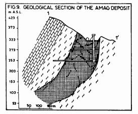
Karstification is mostly developed at crossings of tectonic dislocations. Karst cavities with water and gouge filling have ellipsoid-shaped outlines running in vertical directions and reaching volumes of 100 m<sup>3</sup> and even more.
