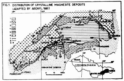
1-Neogene, 2-Paleogene, 3-sediments of the border synclinal structure between the Gemeric and Veporic (Devonian to Upper Carboniferous), 4-Mezozoic of the Gemeric unit, 5-Paleozoic of the Gemeric unit, 6-Veporic unit, 7-nappe overthrust plane, 8-fault, 9-deposit of magnesite
