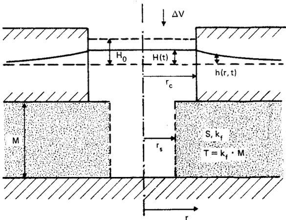
Figure 4: Idealized representation of a finite-diameter well
