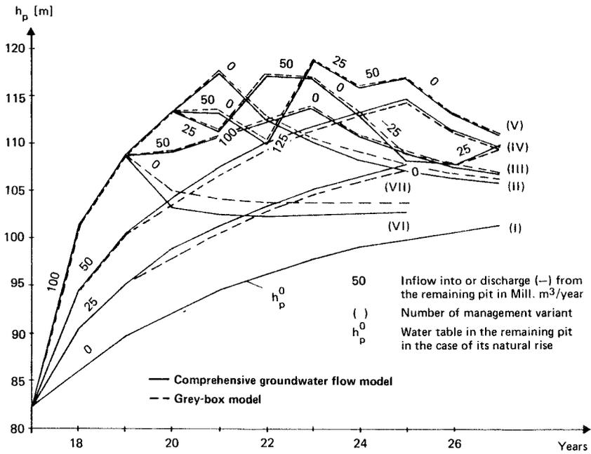
Figure 3: Water table in the remaining pit for different management variants - grey-box model
