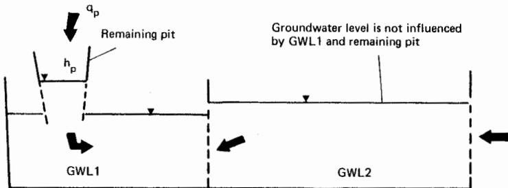
Figure 2: Block structure of the grey-box model
