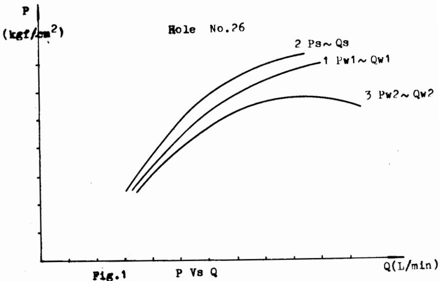
It's proven that water glass injected into ground has a lubrication function to reduce the ground resistance, it also gives the answer on theory why the quantity of cement grout injected can be increased by using pretreatment.
