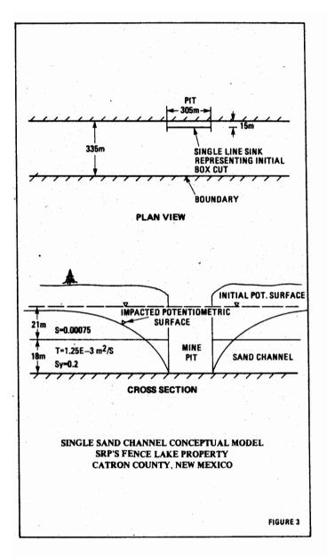
the mine pit penetrating to the bottom of the aquifer. The impermeable boundaries of the sand channel are simulated using the theory of superposition. Image line sinks are placed on the other side of the boundary at the same distance as the real line sink. The initial box cuts of the mine should be opened for two to four months. Inflow to these initial cuts is predicted by the model to be between 1.9E-2 and 3.8E-2 m/s.
