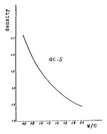
Fig.1 The relationship between the grout density and specific gravity
