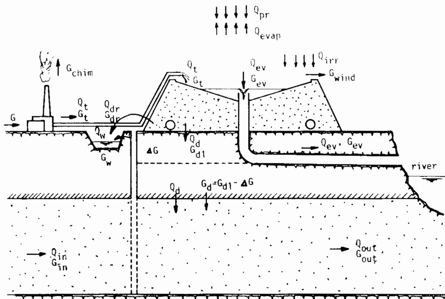
Figure 1: Transport of water and pollutant through the ash depository
