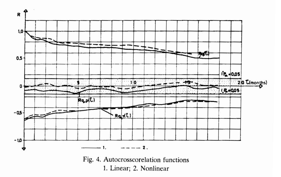
Owing to a marked regularity of inflow and tonnage of the ore recovered, some prognostic dependencies have been established. They can be successfully employed in forecasting the inflow of mine water from one to five months in advance.
