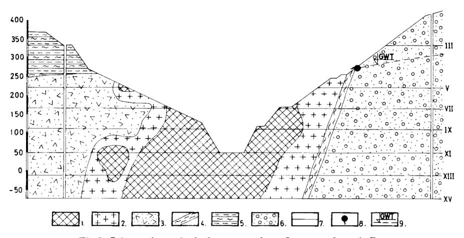
Fig.2. Schematic geological cross-section of copper deposit Bor 1. Ore body; 2. Hydrothermally altered volcanic rocks; 3. Pyroclastic rocks hornblende-biotite andesite; 4. Fault (fault clay); 5. Pelytes; 6. Conglomerates; 7. Working horizon; 8. Spring; 9. Ground water table
