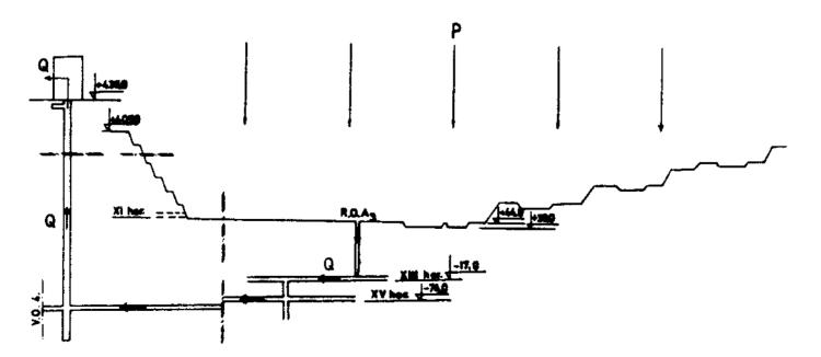
Fig. 3. Schematic illustration of the working mine works in the Bor copper mine P - Precipitation; Q - Mine water
