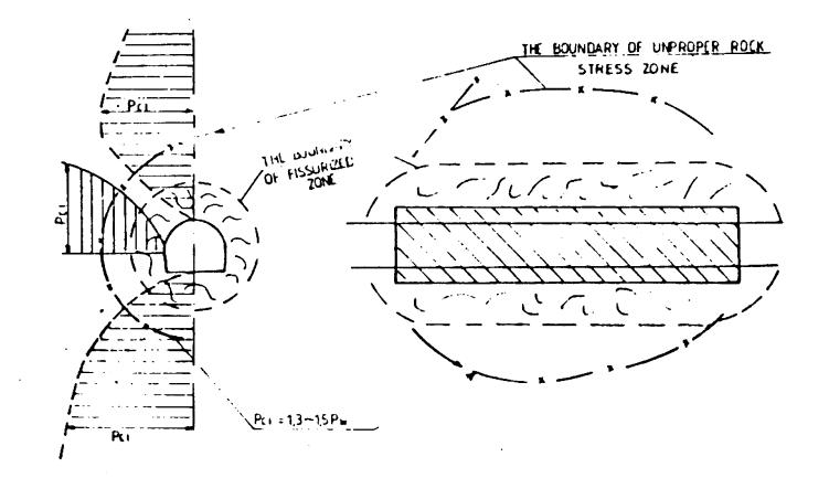
Fig. 2 Zones to be treated around roadways when bulkheads are applied.
