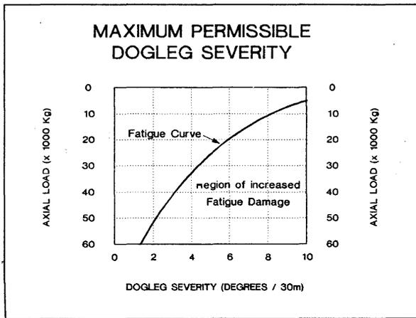
Figure 1.2 Typical fatigue curve for determining Maximum permissible dogleg severity
