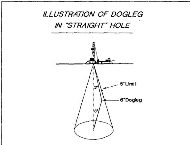
Figure 1.1 Illustrating dogleg severity in "straight" hole
