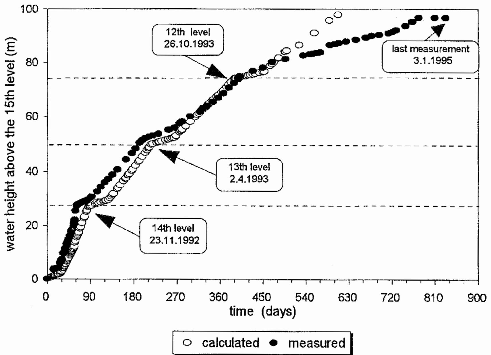
Figure 5: Corrected prognostic curve and measured curve of the water level increase
