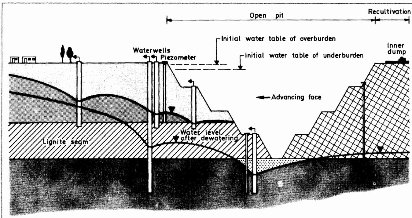
Figure 2. Schematic diagram of dewatering of open pits.
