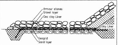
Figure 6. Elongation of the seepage way with geosynthetic liners for avoiding of piping.
