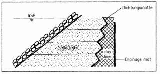
Figure 11. Installation of sealing mats.
