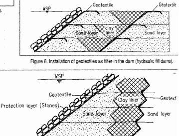
Figure 9. Installation of filtermats behind the core (hydraulic fill dam).
