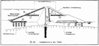
Figure 2. Possible applications of geotextiles in retaining dam construction (DVWK, 1989).
