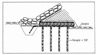
Figure 7. Shows the installation of a horizontal filter with vertical drainage and a geogrid with high tensile strength.
