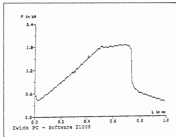
Figure 6. Record of sleeve fracturing.
