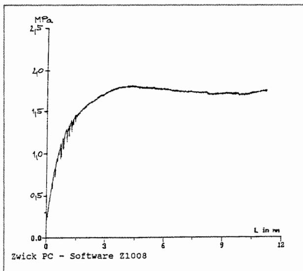
Figure 7. Record of uniaxial compressive strength test.
