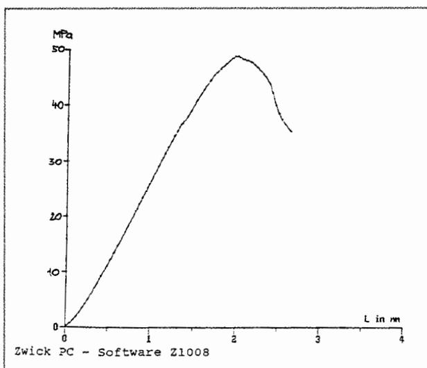
Figure 8. Record of uniaxial compressive strength test.
