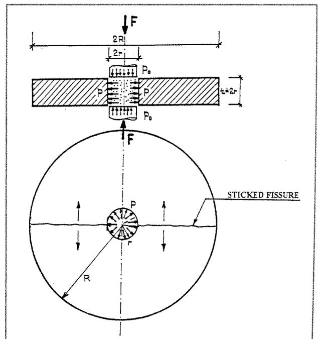
Figure 5. Scheme of adhesive tensile strength - sleeve fracturing test.
