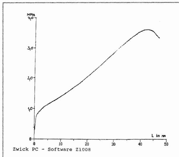
Figure 9. Record of uniaxial compressive strength test.
