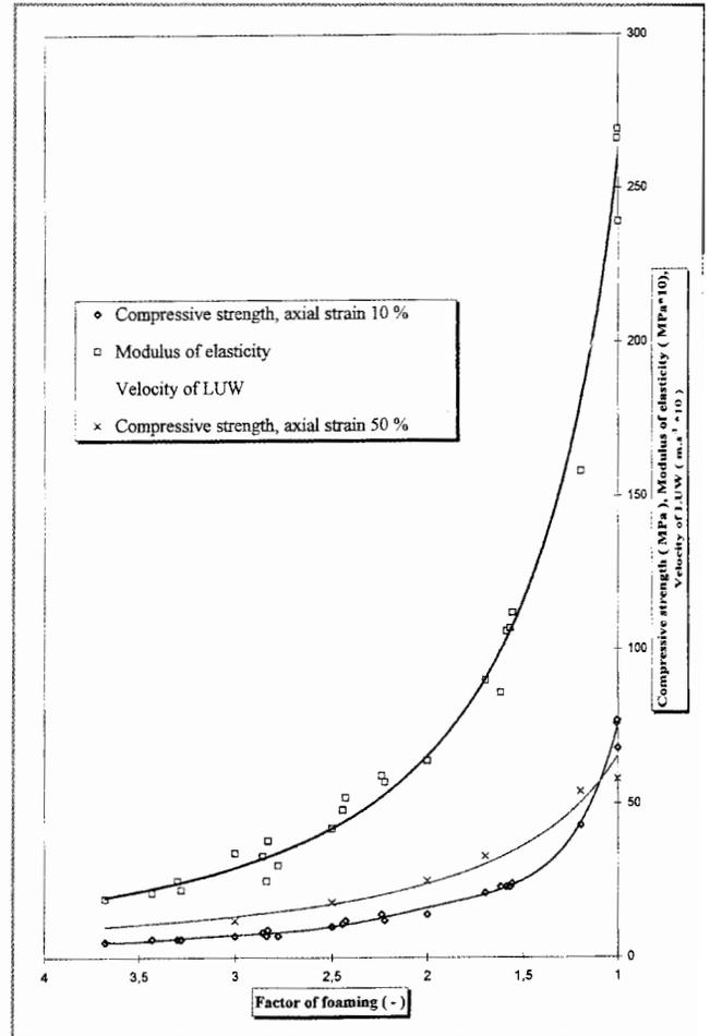
Figure 2. Compressive strength, modulus of elasticity and velocity of longitudinal ultrasonic waves vs. factor of foaming.
