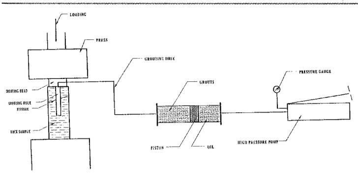
Figure 4. Scheme of fissure grouting test.
