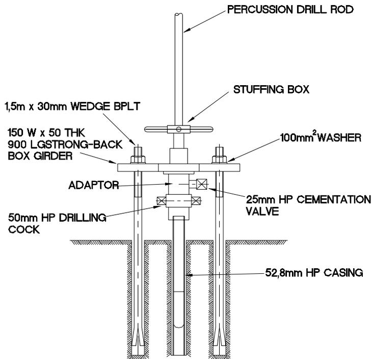
Figure 4 Percussion cover drill casing
