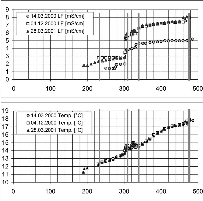
**Fig. 4.** Temperature and conductivity profiles (LF in mS/cm) at monitoring station e-1260 in the mine field of Ronneburg NW. Depth in meters below surface. Grey vertical bars indicating mine levels which are interconnected with the well.
