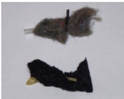
Fig.3. Geotextile used in the Hydrogen Contact Reactor before biofilm formation (top) and after biofilm formation (bottom).
