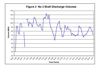
In order to keep the mining basin dry, water is pumped from the underground workings at an average rate of 75 mega litres per day (MI/d). The pumping rates vary seasonally, as shown in Figure 3, between 30 and 120 MI/d historically. Under the current water use license, the mine is allowed to release up to 96 MI/d of HDS treated water.
