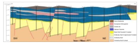
Figure 4. SW - NE cross section through Grootvlei Mine
