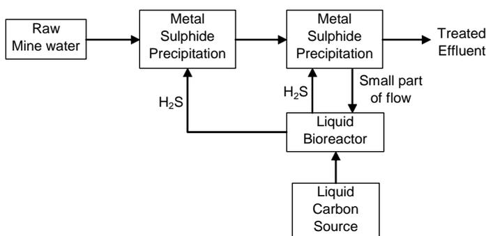
**Fig. 4. Outline of a conceptual liquid bioreactor plant**
