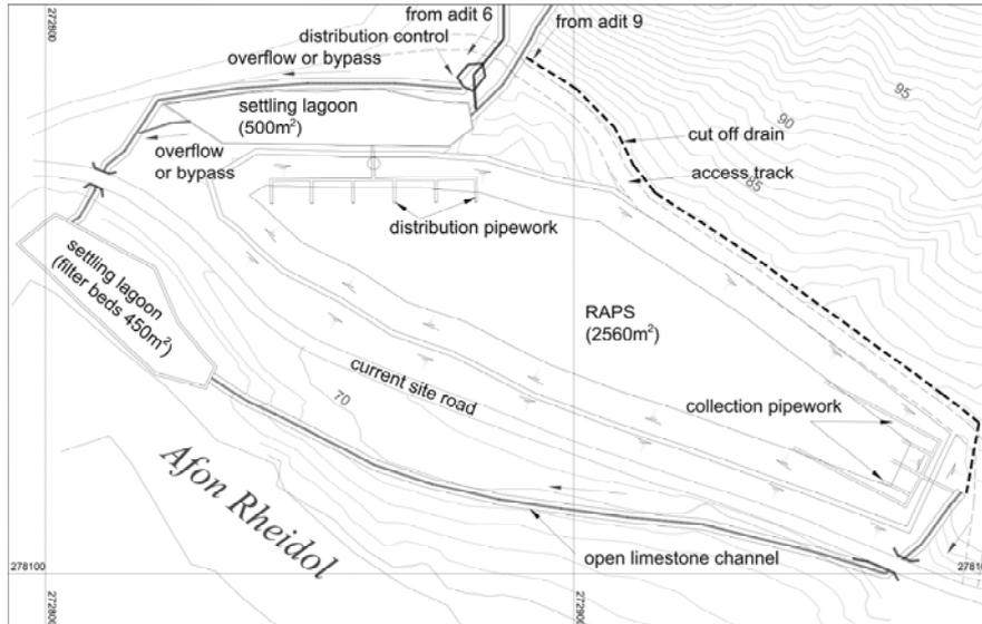
**Fig. 5. Plan of passive treatment system**
