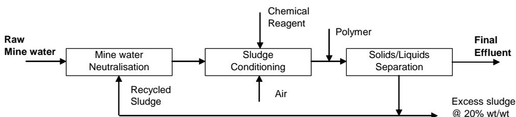
Fig. 3. Outline of a conceptual alkali dosing plant
