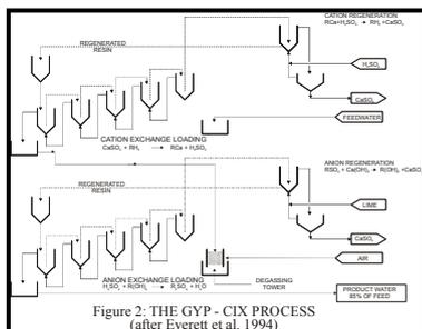
In a pilot plant the effluent of Berkeley Pit, Butte, Montana was treated by the GYPCIX process and the results are given in Table 2. The GYPCIX process can be used to treat solutions with sulfate up to 2000 mg/L and calcium up to 1000 mg/L. Thereafter membrane filtration is required to remove salts.
