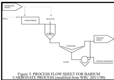
Figure 3: PROCESS FLOW SHEET FOR BARIUM CARBONATE PROCESS (modified from WRC 203/1/90)
