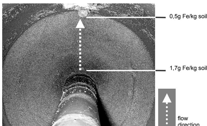
Fig. 7. iron propagation in the grey cast iron injection test
