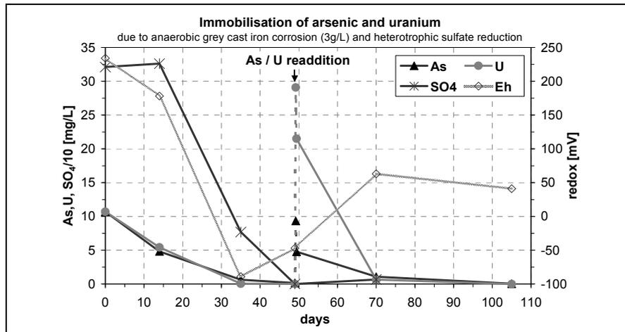
**Fig. 1.** trends of arsenic, uranium, sulphate and redox due to anaerobic grey cast iron corrosion and heterotrophic sulfate reduction
