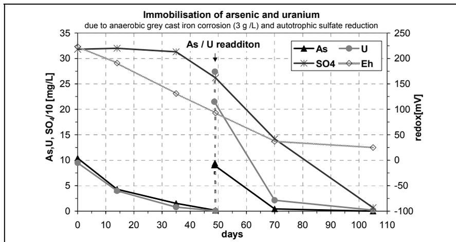
**Fig. 2.** trends of arsenic, uranium, sulphate and redox due to anaerobic grey cast iron corrosion and autotrophic sulphate reduction
