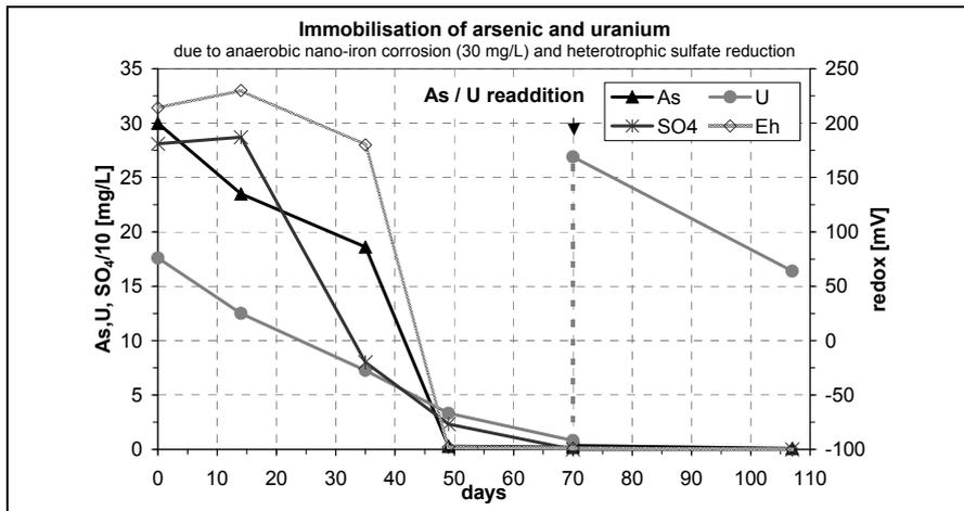
Fig. 3. trends of arsenic, uranium, sulphate and redox due to anaerobic nano iron corrosion and heterotrophic sulphate reduction
