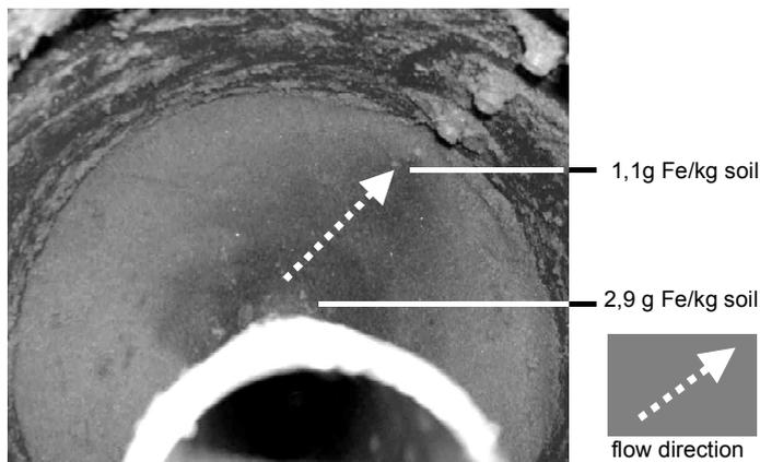
**Fig. 6.** iron propagation in the nano scale iron injection test
