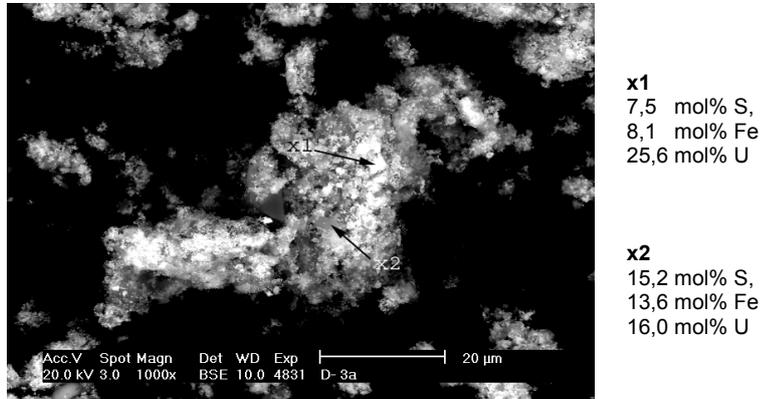
**Fig. 5.** SEM micrograph and EDX analysis of iron precipitate from an attempt with nano scale iron and heterotrophic sulphate reduction
