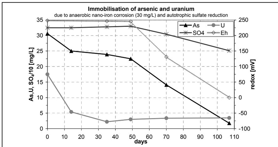
Fig. 4. trends of arsenic, uranium, sulphate and redox due to anaerobic nano iron corrosion and autotrophic sulphate reduction
