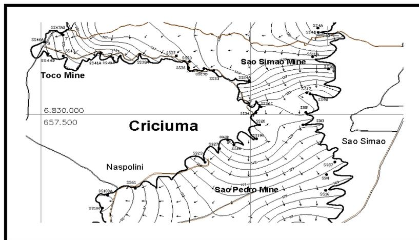
**Figure 03: Map showing structural model of Barro Branco coal seam floor and flow directions inside the mines.**
