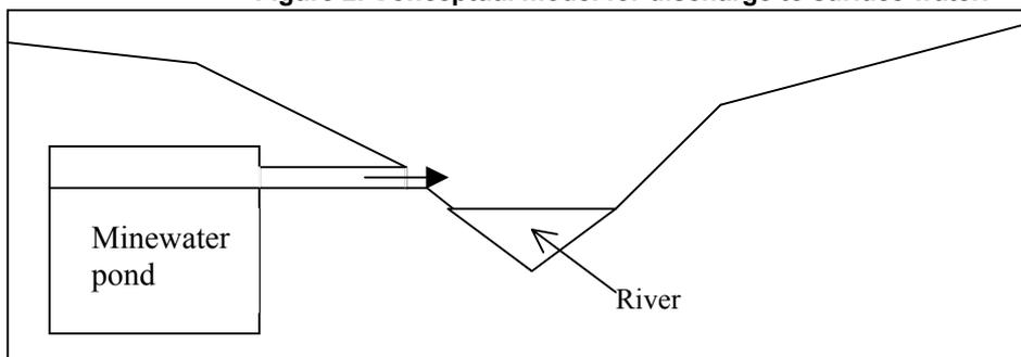
The flows calculated by GRAM for the Treeton and Silverwood ponds (Table 1) are mixed with the flow in the River Rother and River Don. PHREEQC was applied as a batch-reaction model by taking the volume of flow in a fixed time period (e.g. 1 second) and mixing the two waters together. It was assumed that the minewater and river water completely mix, and that equilibrium was instantaneous. It is recognised that both these assumptions are simplifications but are deemed appropriate for this study.
