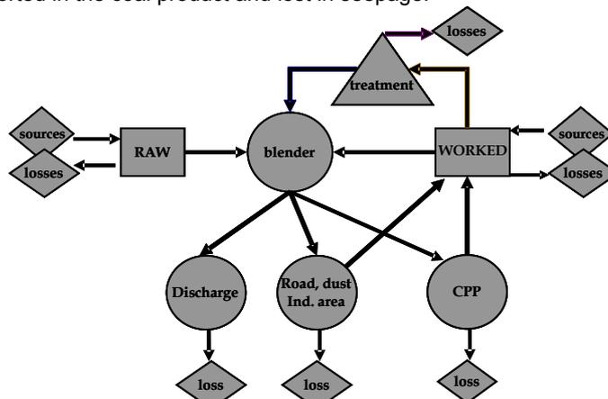
**Figure 1. System diagram of a simple coupled salt and water balance model for a mine site (circles represent water using processes, rectangles are stores and diamonds losses and sources of water/salt).**
