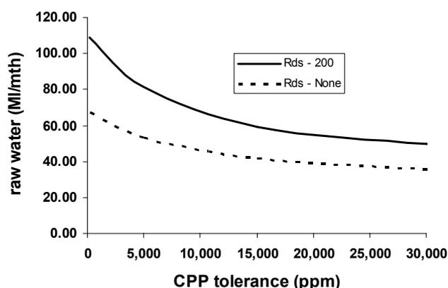
**Figure 2. Raw water use with increasing salt tolerance in CPP for the case of no salt constraint for road water watering and raw water (200ppm) required for road watering.**
