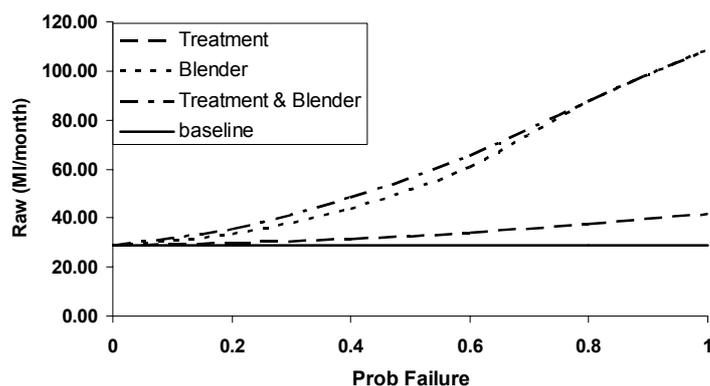
Figure 5. The effect of blender failure compared to treatment failure (treatment is 0.6 MI/d).
