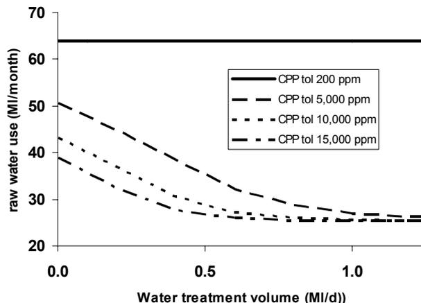
**Figure 3. Raw water use with increasing water desalination volume, for a range of CPP salt tolerances.**
