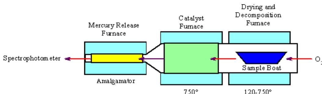
Figure 1: Schematic diagram of the mercury specific analyser DMA-80
