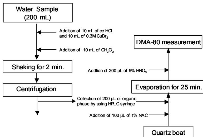
Figure 2: Extraction method for the determination of the organic mercury fraction
