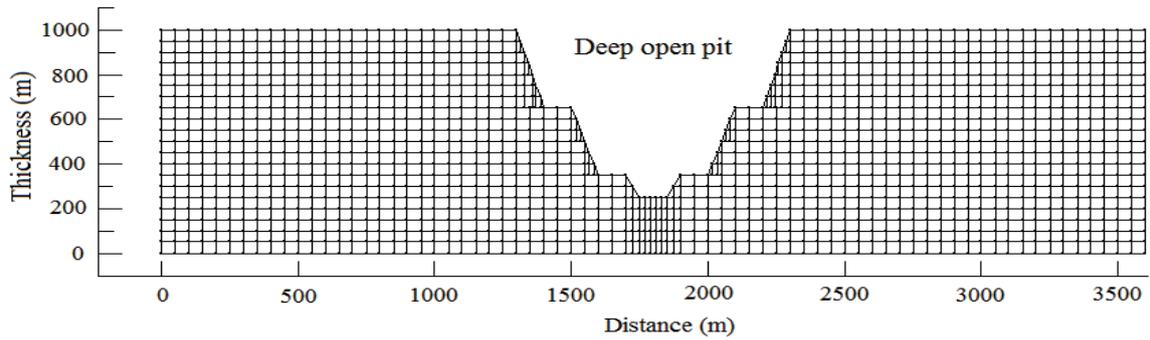
Figure 2. Finite element mesh for a deep open pit in an unconfined aquifer.
