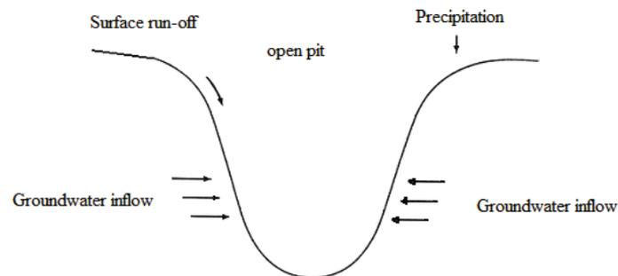
Figure 1. Inflow components into an open pit.
