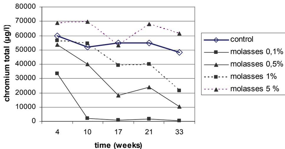
Figure 2. Evolution of total Cr concentrations in groundwater in mesocosms after inducing a reduced environment by adding molasses at different concentrations.
