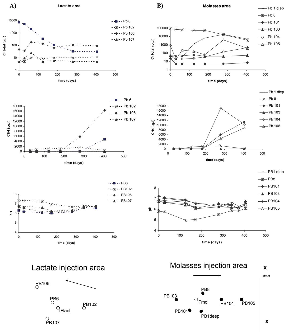
**Figure 4. Schematic representation of the impact zones of lactate injection (A) and molasses injection (B) presenting results of total [Cr], methane and pH. Filter depths are as follows for lactate zone: Pb6: 4.1 m bg; Pb102: 7.2 m bg; Pb106: 4.2 m bg; Pb107: 6.2 m bg, injection filter (IF): 0.5 – 12 m bg. Filter depths for molasses zone are: Pb1 deep: 11.0 m bg; Pb8: 3.0 m bg; Pb101: 8.5 m bg; Pb103: 6.2 m bg; Pb104: 5.0 m bg; Pb105: 6.2 m bg; IF: 0.5 – 12 m bg.**
