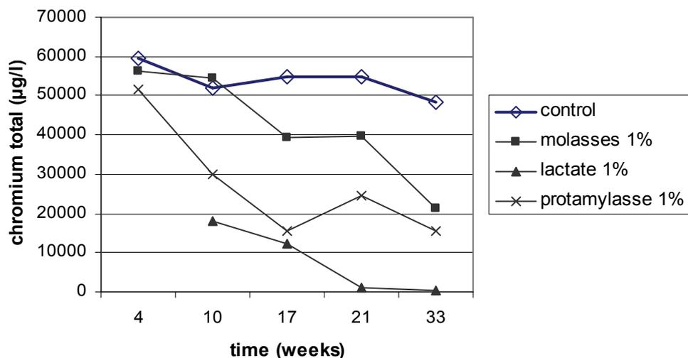
Figure 3. Evolution of total Cr concentrations in groundwater in mesocosms after inducing a reduced environment by adding different substrates (1% Carbon source).
