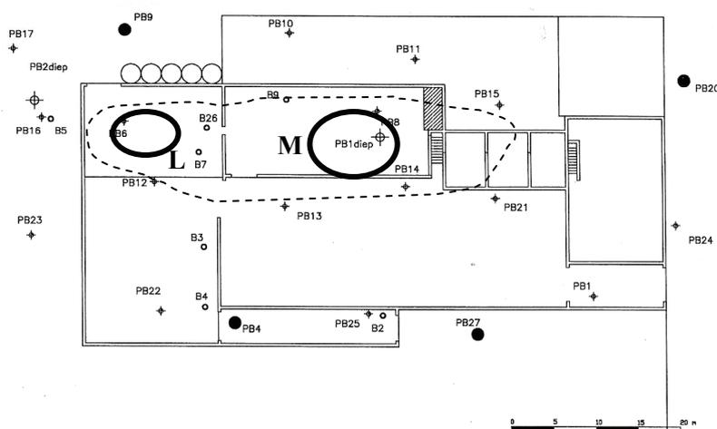
**Figure 1. Chromium(VI) plume in the groundwater at an industrial site in Flanders. Black ellipses indicate the areas of pilot scale test for Lactate (L) and Molasses (M).**
