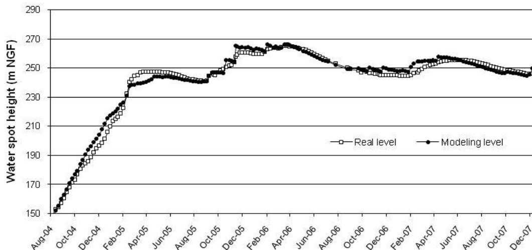
The curve gives an indication of the reliability of the model: 93% of the calculated levels are within +/- 7 m of observed values. The standard deviation between the curves is 3.5 m with an average variation of 0.97 m. Despite its simplicity the model predicts the water fluctuations in the mine quite well, using only the three input/outflow parameters discussed earlier. This result allows us to put aside the possibility of other significant inputs and outflows.
