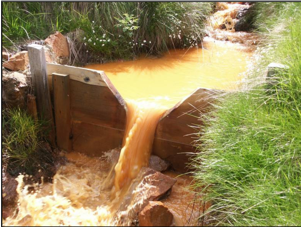
Figure 3 The representation of the measuring of the abundance of mining waters at the Thompson's weir
