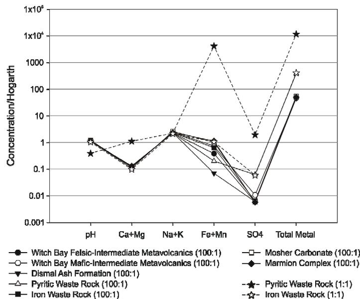
**Figure 3** Sulfur concentrations of reaction column experiments for water quality prediction upon outflow in 2030-2060. MTR is the minimum toxic response based on non-rock buffered mixing experiments (see Table 1).
