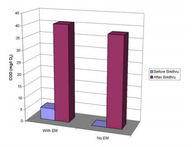
Figure 4. Influence of engineered microbes on COD before and after breakthrough
