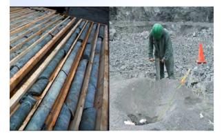
Post-blast waste rock monitoring is needed to check if sulphides preferentially report to waste rock fines. In this example, post-blast monitoring indicated the preferential accumulation of AP was 2x higher than NP in < 2 mm particles of a volcanic waste rock.
