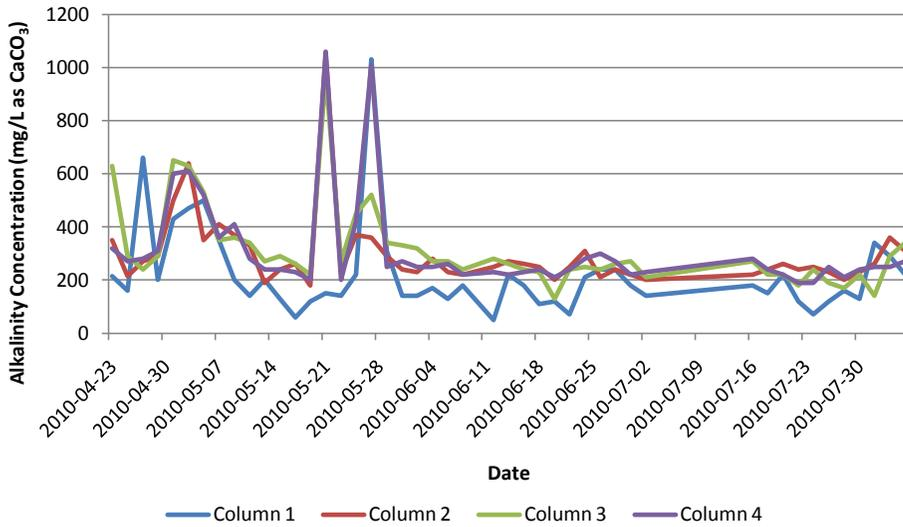
Figure 2 Alkalinity concentration in the effluent of each column. Column 1: mixed wood chips and slag, Column 2: mixed river gravel and slag, Column 3: slag, Column 4: layered wood chips and slag
