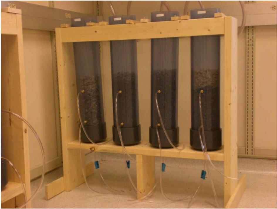
*Figure 1* Laboratory column setup. Columns contain 1) 20% wood chips mixed with 80% slag, 2) 20% river gravel mixed with 80% slag, 3) 100% slag, and 20% wood chips layered on top of 80% slag
