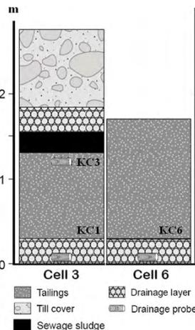
**Table 1** Original chemical composition of tailings and sludge in 2001 (- indicate no analysis) **Figure 1** Profiles of the two cell cover pilot-scale experiments with reference to leachate probes
