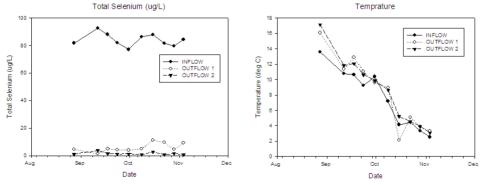
Figure 1 Selenium removal as a function of temperature at Smoky River Coal
