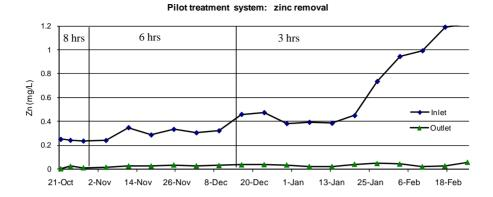
*Figure 2* Dissolved zinc concentrations in a bioreactor operated at different retention times and zinc loadings
