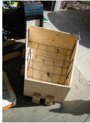
Figure 3 View of the assembled bottom portion of the mould, wire mesh and rebar handles.
