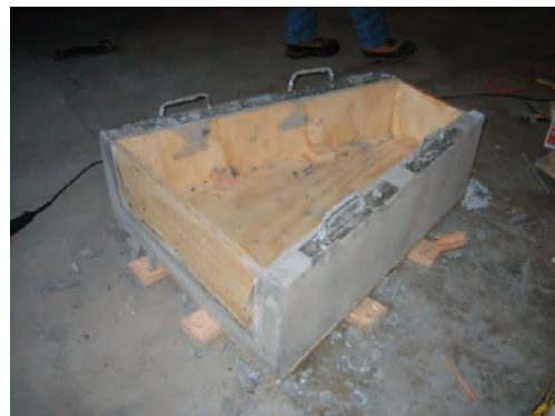
Figure 4 View of the curing concrete; mould bottom is removed.
