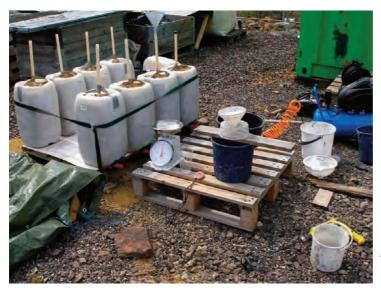
*Figure 1* Small pilot trials (25 L) with the plastic pipes for injection.
