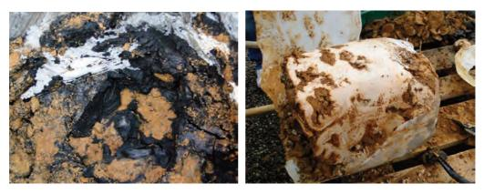
**Figure 4** Deconstruction of 25 L pilot trials. Injection with green liquor dregs (left) indicate that all voids have been filled and that impermeable layers have been formed. Mine waste injected with lime kiln dust (right) has formed a solid unit with very low permeability.
