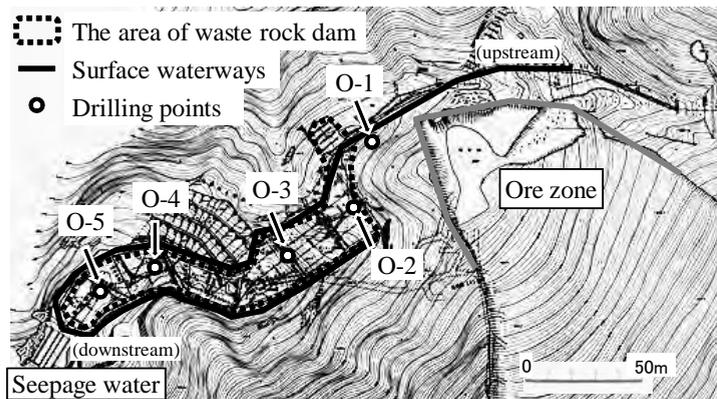
Figure 4 Waste rock dam of O mine
