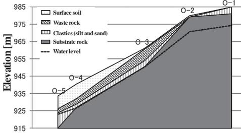
**Figure 7** Geological section of the waste rock dam at O mine
