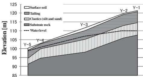
**Figure 5** Geological section of the tailing dam at Y mine
