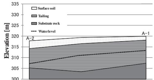
**Figure 6** Geological section of the tailing dam at A mine
