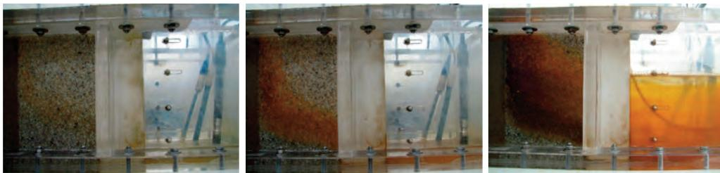
**Figure 3** Front view of the outflow chamber with the well screen section, gravel pack and aquifer material (from the left to the right of each picture; height: 200 mm). Progress of incrustation growth at 0 h (left), 17.5 h (middle) and 123.0 h (right) after the first breakthrough of Fe(II) through the flow channel.
