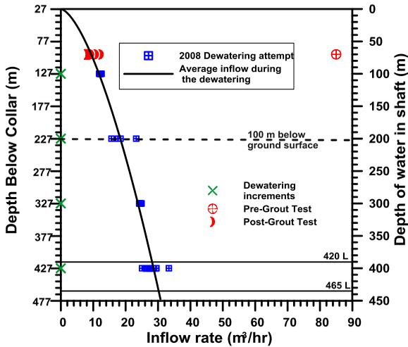
Figure 3 Flow rates for the 2008 dewatering.
