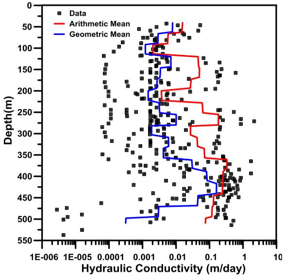
Figure 1 Variation of hydraulic conductivity with depth.
