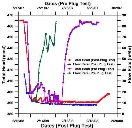
Figure 2 Results from pre and post plug tests
