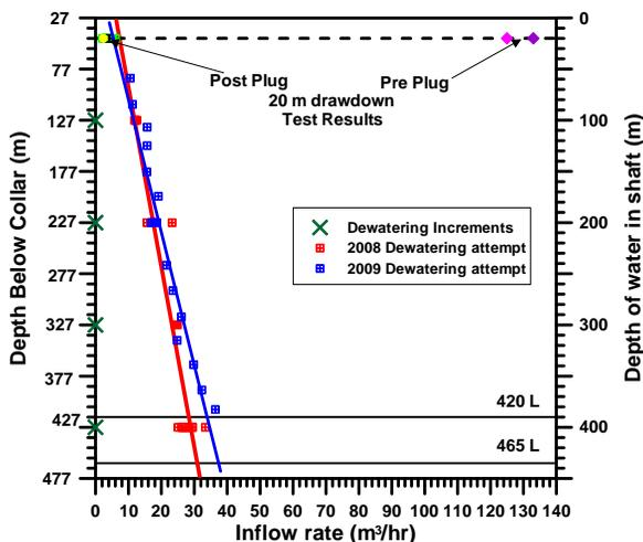
Figure 8 Data for 2008 inflow remediation and 2009-2010 dewatering
