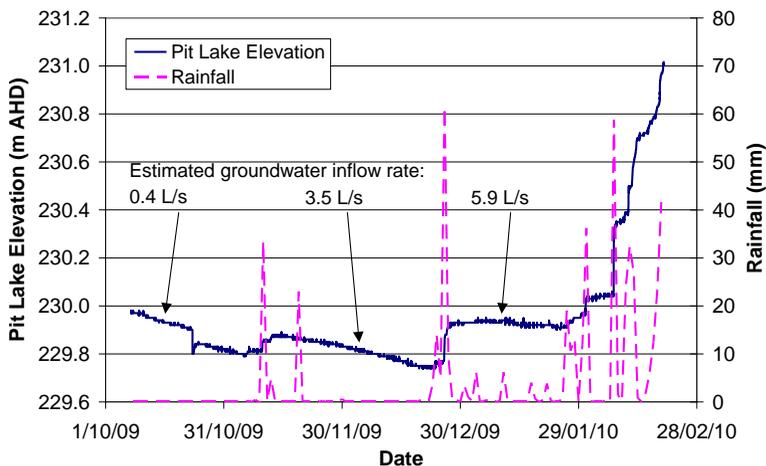
**Figure 9:** Groundwater inflow estimation for pit
