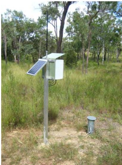
**Figure 5:** Groundwater bore monitoring station
