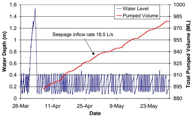
**Figure 7:** Dam seepage inflow derivation – Plumtree Creek Dam
