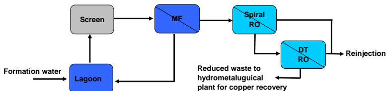
**Figure 4** Process flow block diagram of copper mine water processing system
