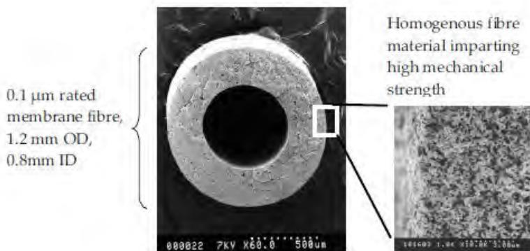
**Figure 2** PVDF Hollow fibre filtration membrane
