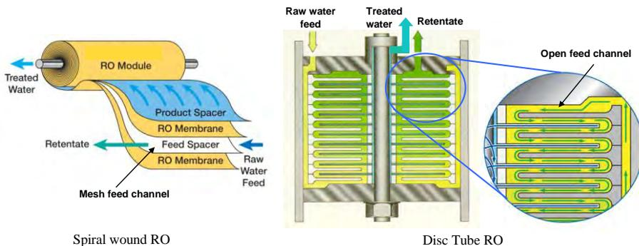
**Figure 3** RO module configurations
