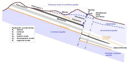
*Figure 1* Groundwater conditions in a coal bearing sequence (modified after Thomas 2002)
