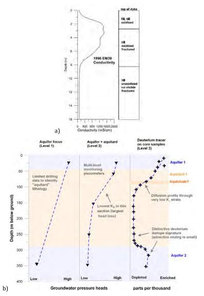
**Figure 2** a) Geophysical logging to detect base of oxidized fractured zone in glacial till at a potash mine (Timms and Hendry, 2003) b) Conceptual schematic of information provided by Level 1-3 aquitard assessment
