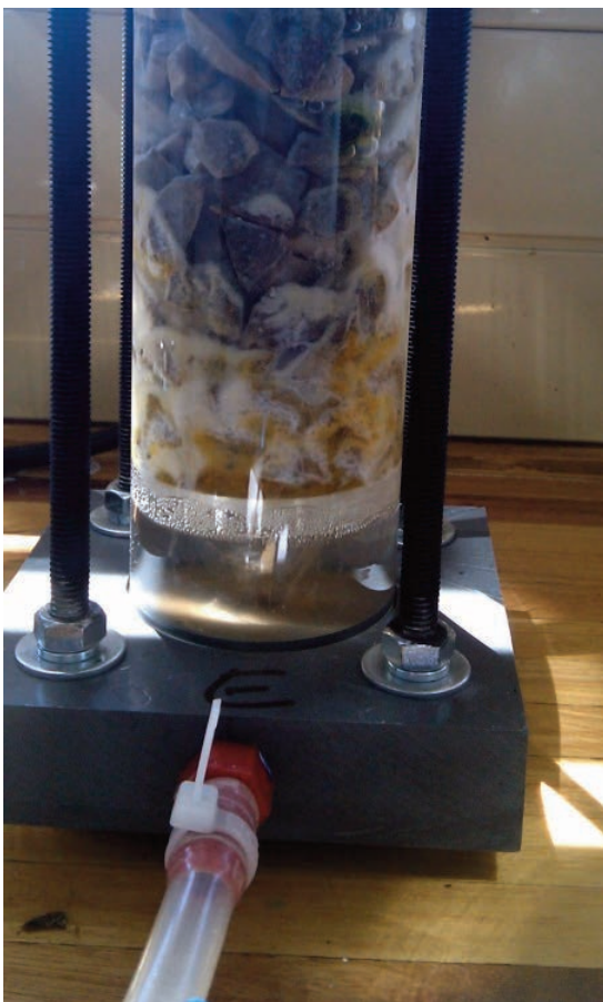
Fig. 4 Precipitate forming at the bottom of a column due to the reaction between synthetic AMD and dolomite.
