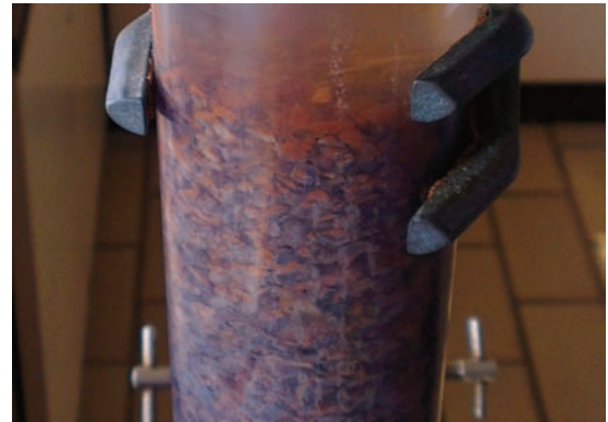
Fig. 6 Iron-rich precipitate in a dolomite-filled column fed with lab-generated AMD
