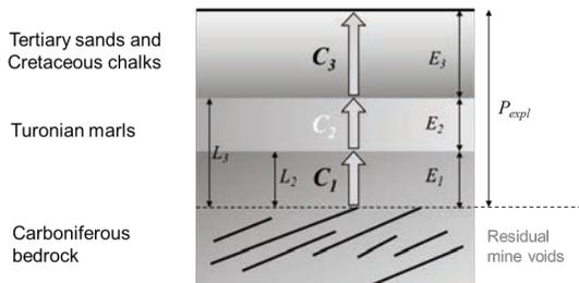
**Fig. 3** Definition of the variables needed to compute specific hydraulic conductance.
