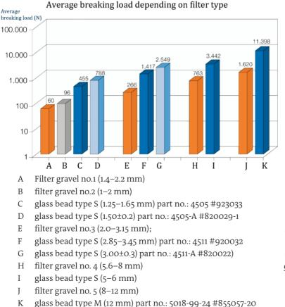
Fig. 3 Magnitudes of break*ing loads for filter gravel* and glass beads at different granulations and bead sizes and mixtures at static load handling (TRESKATIS et al. 2010)
