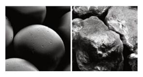
Fig. 2 REM image of a glass bead compared to a filter gravel grain of the same grain size. The "smooth" surface of the glass bead prevents the formation of tensile stress whenload is applied and reduces the agglomeration of incrustations (Treskatis et al. 2010).
