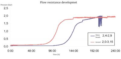
**Fig. 4** Pressure development in gravel packs 2.0 – 3.15 mm grading and glass beads packs grading 2.4 – 2.9 mm under continuous perfusion with iron and manganese containing groundwater more than compensate the initial higher investment.
