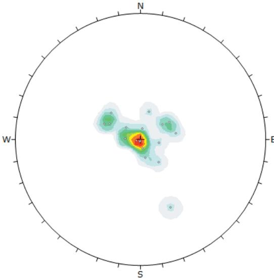
**Fig. 3** Density concentration of poles of structures detected as inflows. A darker colour indicates a higher concentration. Sample size was 21.
