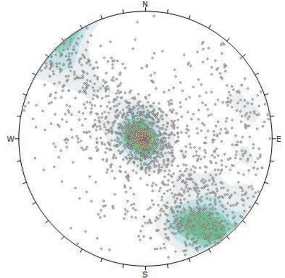
**Fig. 4** Density concentration of poles of all logged structures. A darker colour indicates a higher concentration. Sample size was 3103.
