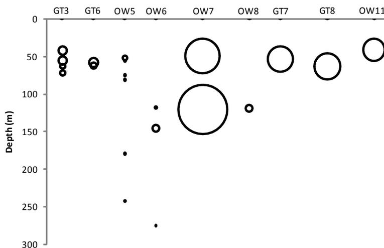
**Fig. 2** Inflow magnitude and depth in each borehole. Each circle represents an inflow. Circle area reflects inflow transmissivity, which has been normalised to the highest transmissivity value in the dataset.
