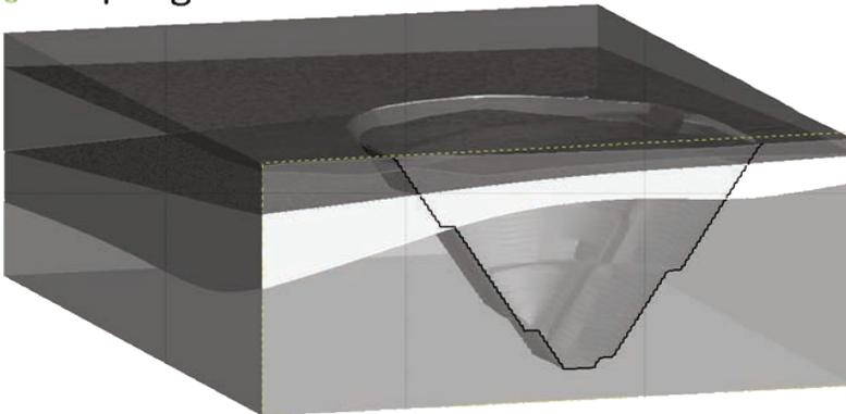
**Fig. 5** Conceptual model block diagram of proposed pit shell with zone in which inflows were detected in white. Weathered zone is dark grey and the remaining rock mass is pale grey. Aspect is towards the north-east and the pit diameter at the line of cross-section is approximately 1km.
