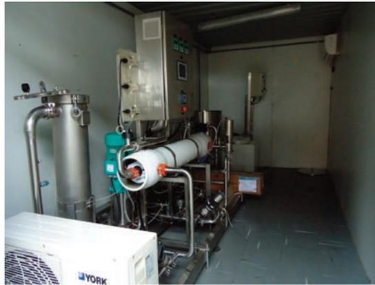
**Fig. 5** Nanofiltration System
