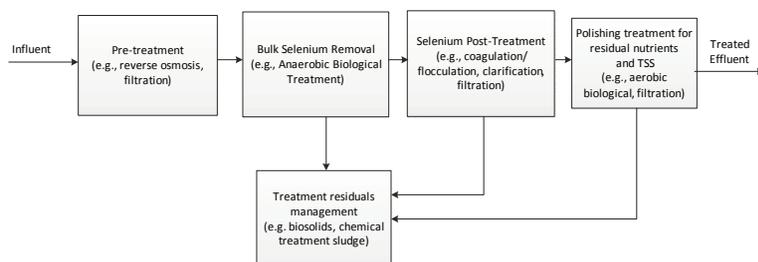
**Fig. 1** Block flow schematic for selenium treatment
