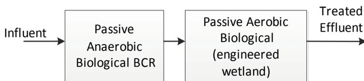
**Fig. 4** Block flow schematic for passive treatment
