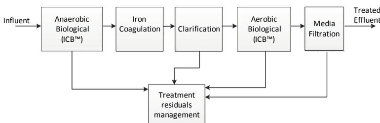
**Fig. 3** Block flow schematic for Case Study #2
